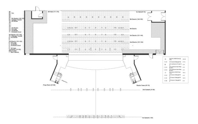
1-4E Circuits are located on 2 x 5 unit Movable Circuit Boxes. These circuit boxes must remain on  $4^{th}$  Electric to maintain Standard Rep Plot.
